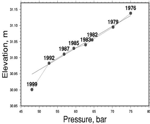
Figure 4. Elevation at a bench mark SN-H2 within the borefield at Svartsengi and pressure in boreholes at 900 meters depth within the reservoir.
