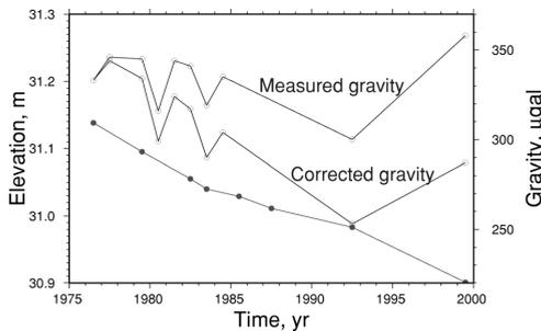
Figure 1. Elevation (filled circles) and gravity variation with time at benchmark SN-H2, located within the borefield at Svartsengi geothermal plant
