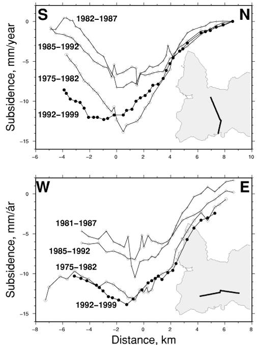
Figure 2. Subsidence rate along NS and EW profile crossing the geothermal field at Svartsengi (at 0 km distance), for four different time intervals
