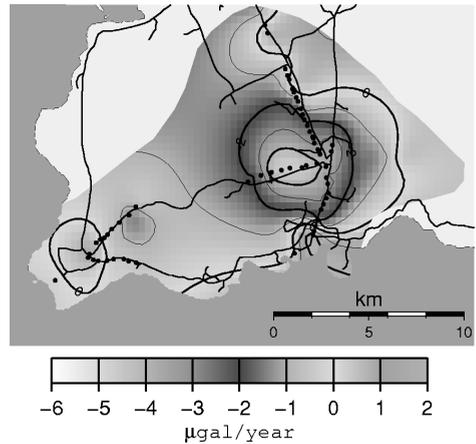
Figure 5. Mean gravity variation ( $\mu\text{gal}/\text{year}$ ) from 1975 to 1999. Only points measured in 1999 and at least two times earlier are used.
